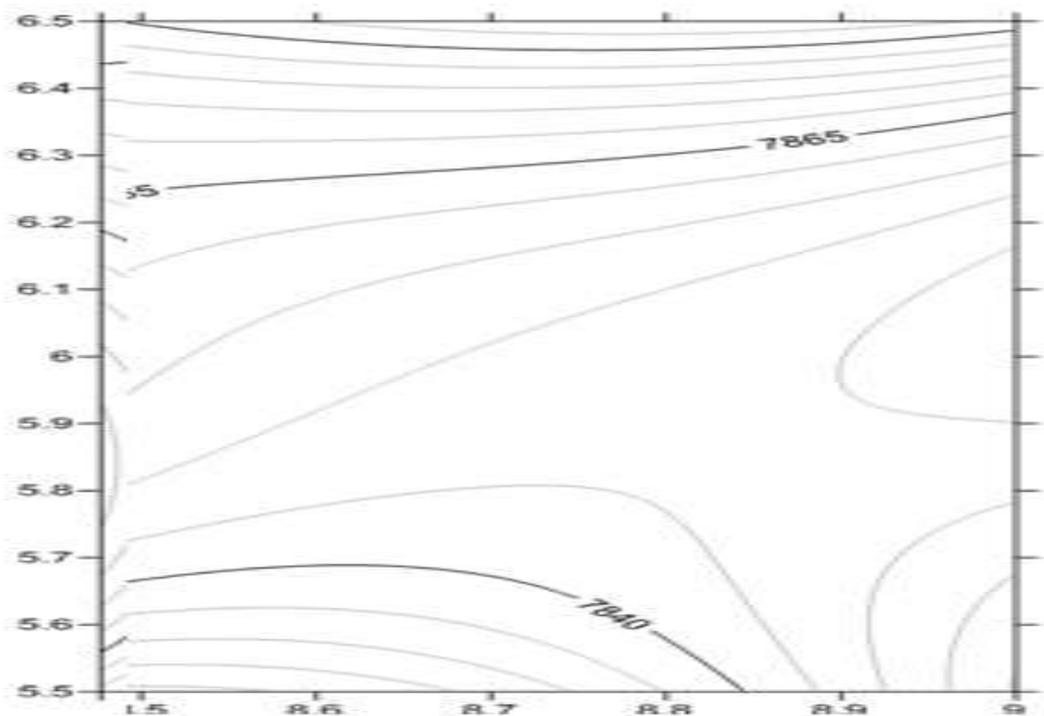
Fig. 6 Third Degree Regional Field of the Total Magnetic Intensity of the Study Area
