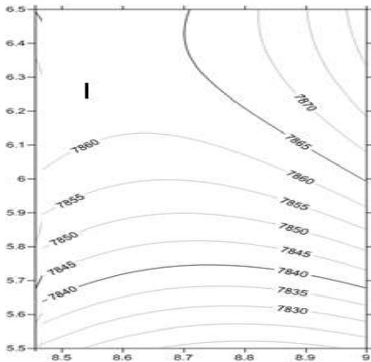
Fig. 5 : Second Degree Regional Field of the Total Magnetic Field of the Study Area
