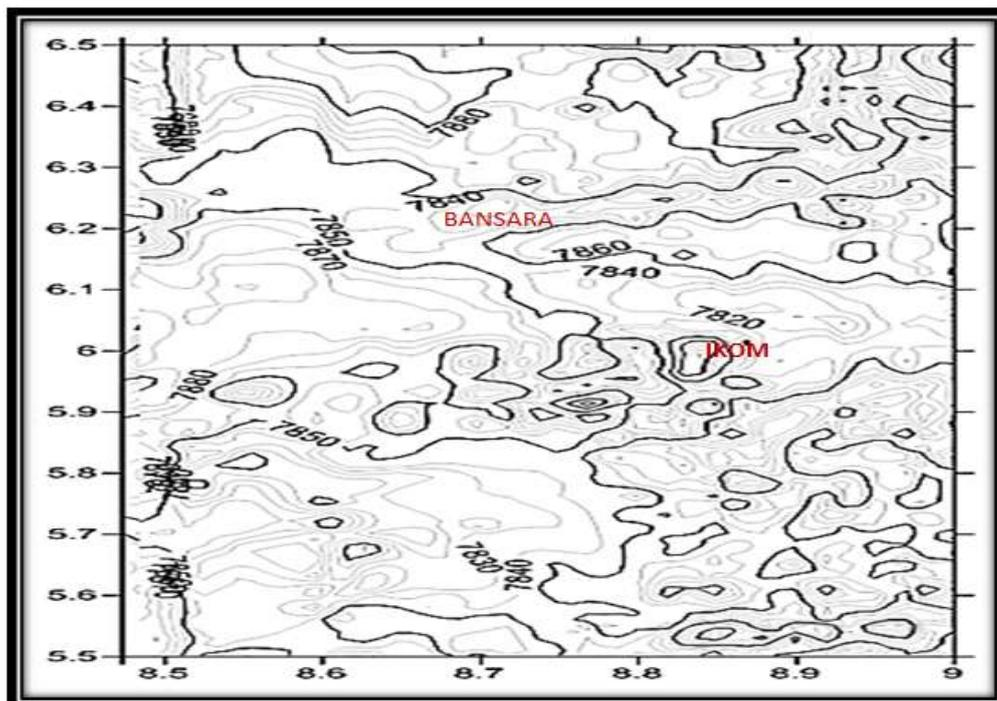
Fig. 2 Total field magnetic intensity contour map of the study
