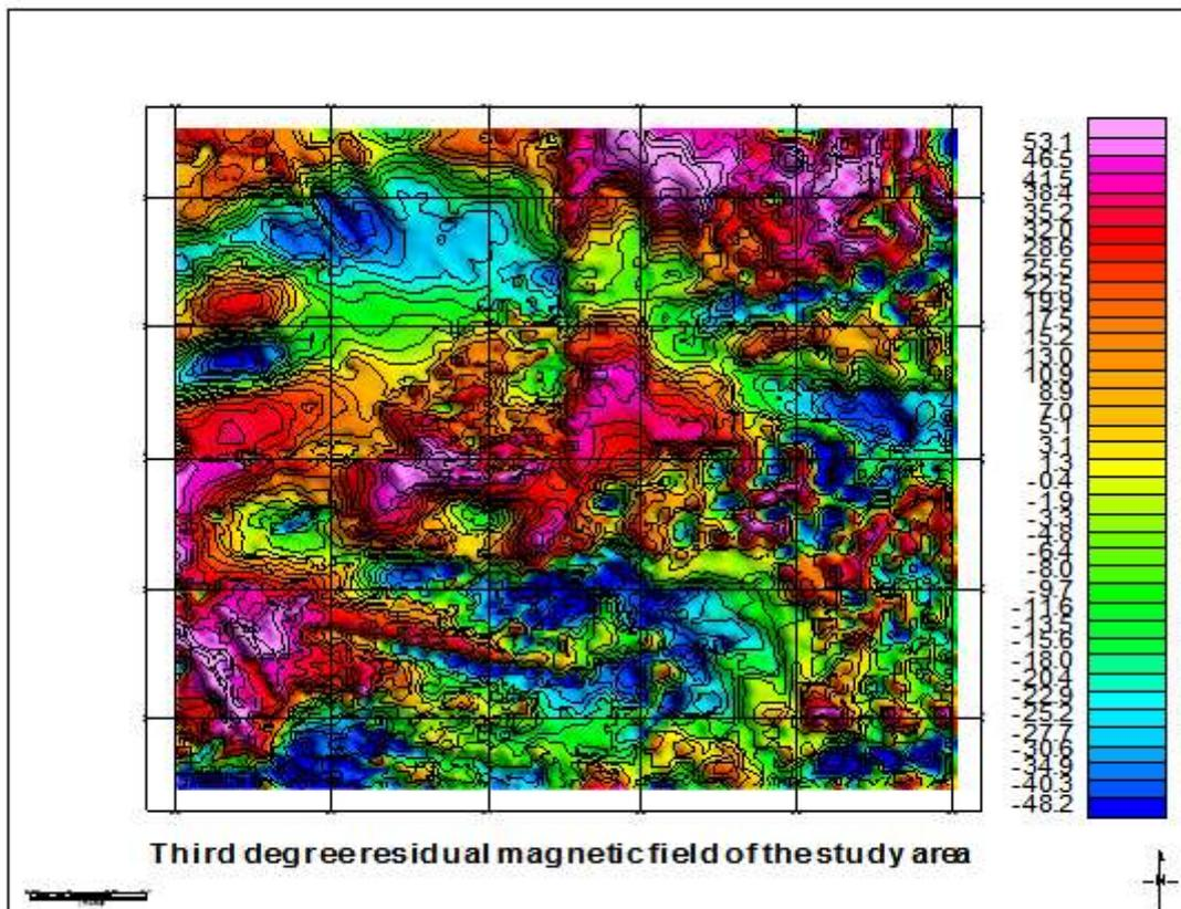
Fig.14 : Third degree residual magnetic field of the study area
