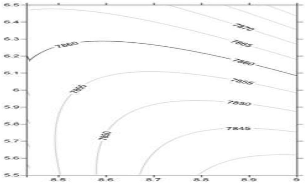
Fig. 7: Fourth Degree Regional Field of the Total Magnetic Intensity of the Study Area
