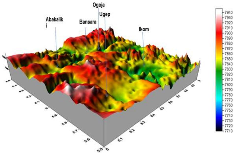
Fig 3 3-D Image of the total magnetic field intensity of the study area
