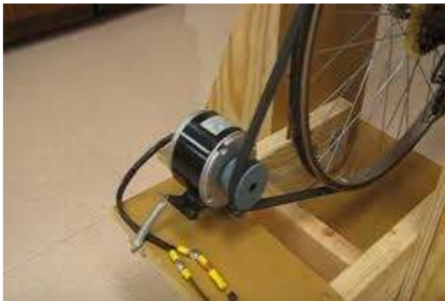
Figure3: Wooden Stand of bicycle generator
