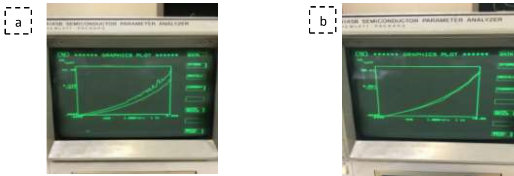
Figure 12: Electrical Properties of RGO-FET devices. I_{ds} - V_{ds} output characteristics of the R-GO FET device with \frac{W}{L} = 10 electrodes. a) The gate voltage ( V_g ) is varied from 0 to 0.4 V with an interval of 0.2 V. b) The gate voltage ( V_g ) is varied from 0 to 0.7 V with an interval of 0.1 V.
