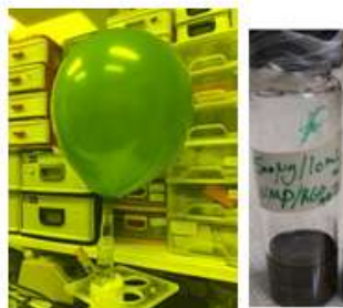
Figure 4: a) The process of activating the surface (Si/SiO 2 /Cr markers/Piranha) with APTES solutions. b) Reduced graphene oxide suspension.
