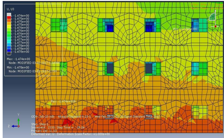
Fig. 20: Deformed shape U_3 at the max. Displacement
