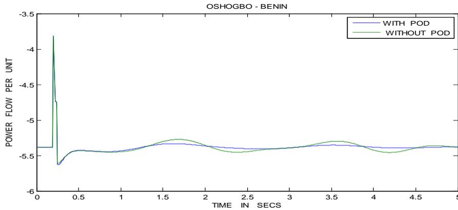
**Figure 11:** Power Flow on Oshogbo-Benin Line
