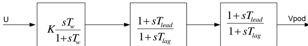
**Figure 4:** POD Block Diagram
