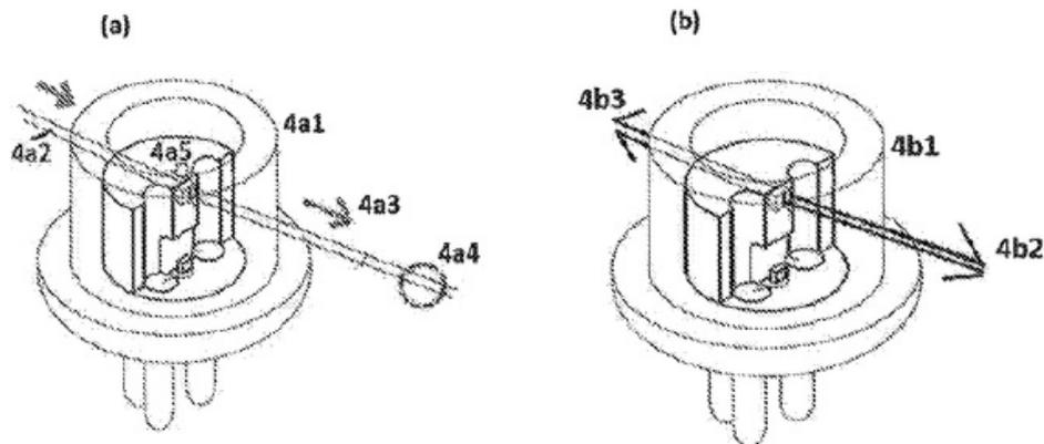
**FIG. 4.** Diagram of the device in which is shown the projection of the induction of forces in external objects (frame 4a) and the possible thrusting in the laser diode structure caused by the self induction of forces (frame 4b).
