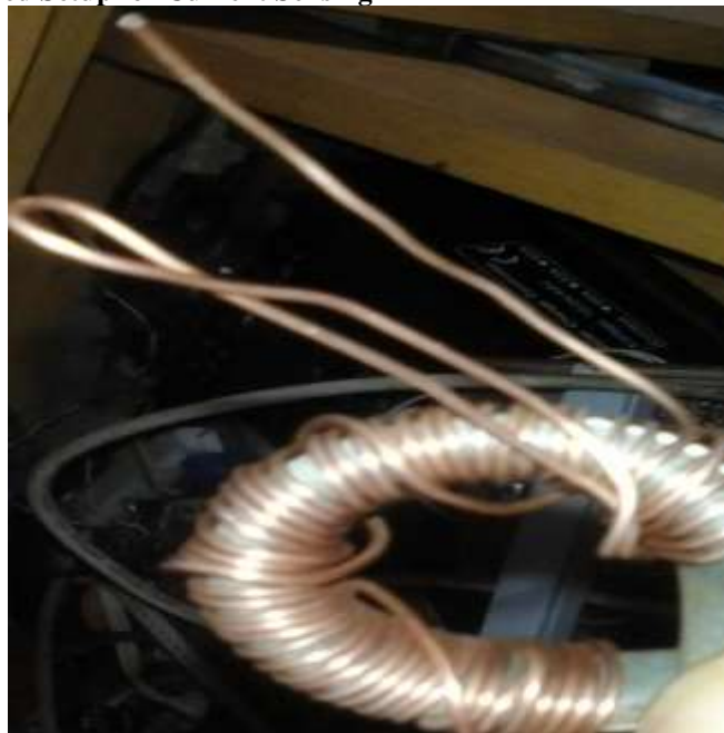
Figure 13 Snapshot of Rogowski Current Sensor as it is wound
