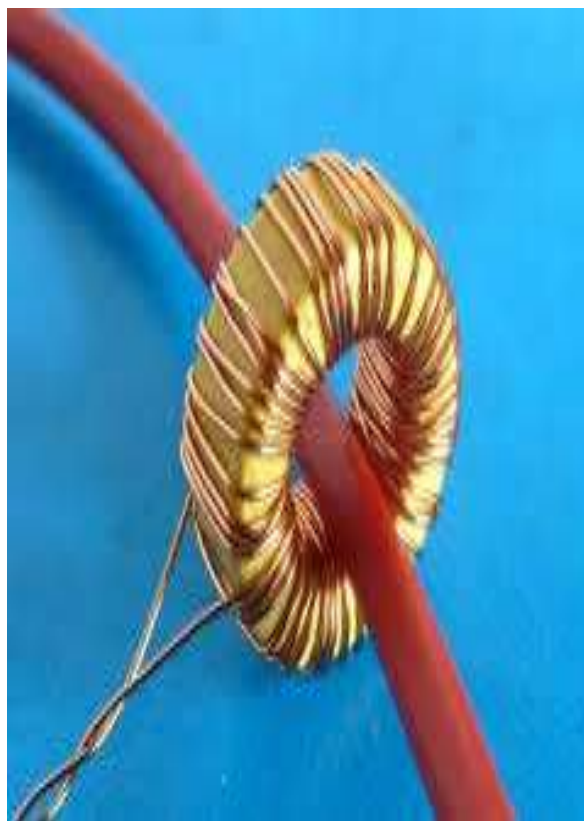
Figure 15 Snapshot of an experimental test-bed set up for a current transformer
