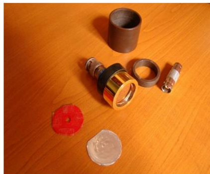
Fig. 2: The special positioning device. Fig. 3: {}^6\text{Li} + Si detector
