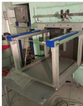
Fig. 2: The special positioning device. Fig. 3: {}^6\text{Li} + Si detector
