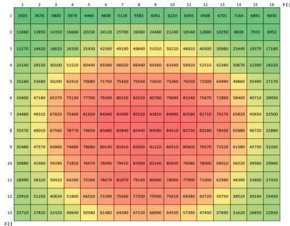
Fig. 5: The intensity distribution of the neutron flux (x = 0 cm).
