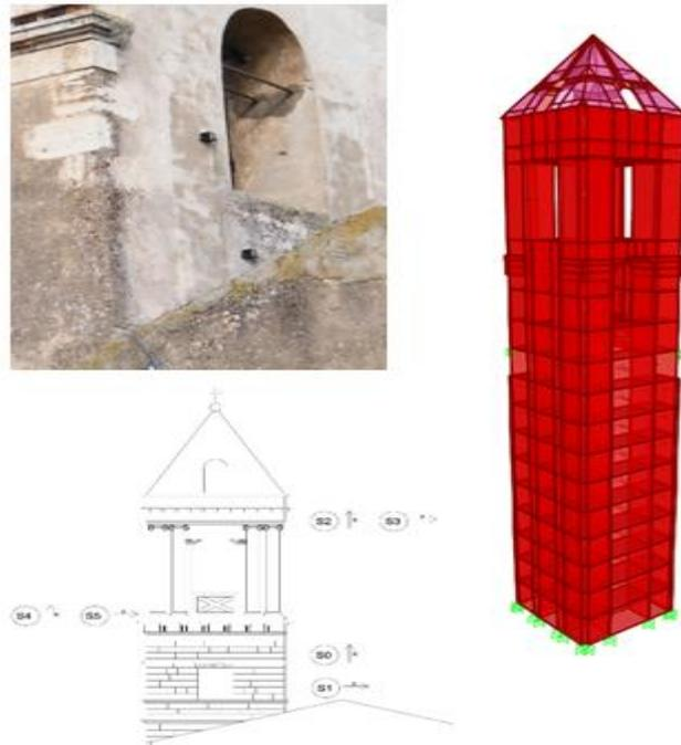
Figure 4: Location of the vibration sensors Figure 5: Finite element model
