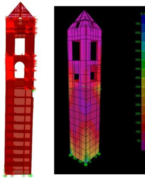
**Figure 9.** Compression stresses due to seismic load ( $\text{daN/cm}^2$ ).  $\text{PGA} = 0,07g$ ;
