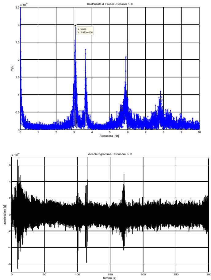
Figure 6: Fast Fourier transform and recorded signal. Accelerometer 0.
