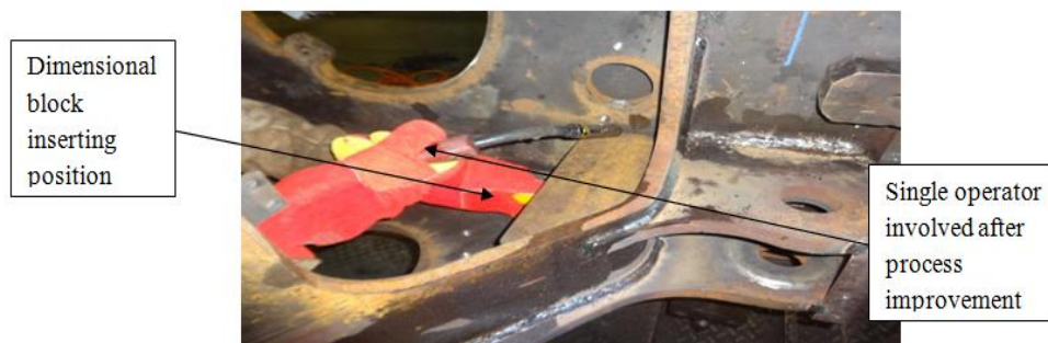
Figure (8) Dimensional block inserted inside plate after process improvement
