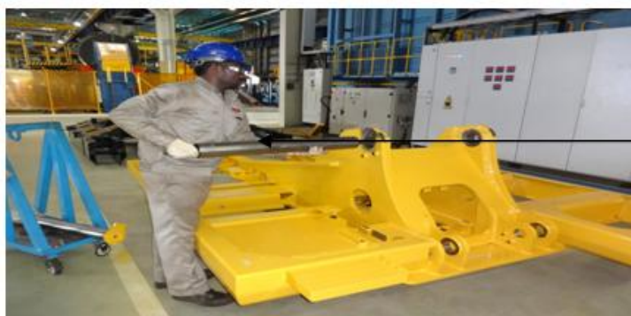
Figure (10) Inline checking of Revo frame after process improvement
