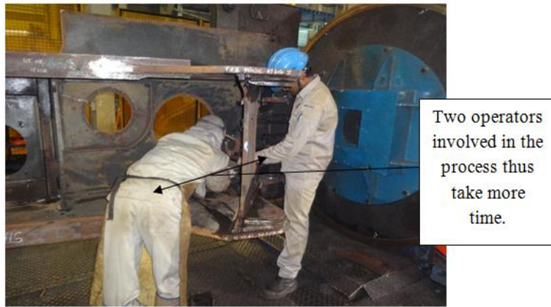
Figure (5) Before process improvement two operator involved
