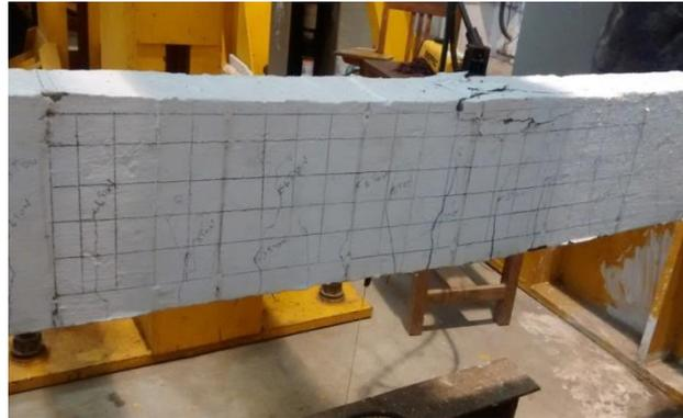
Fig. 6 Failure mode of beam CC1
