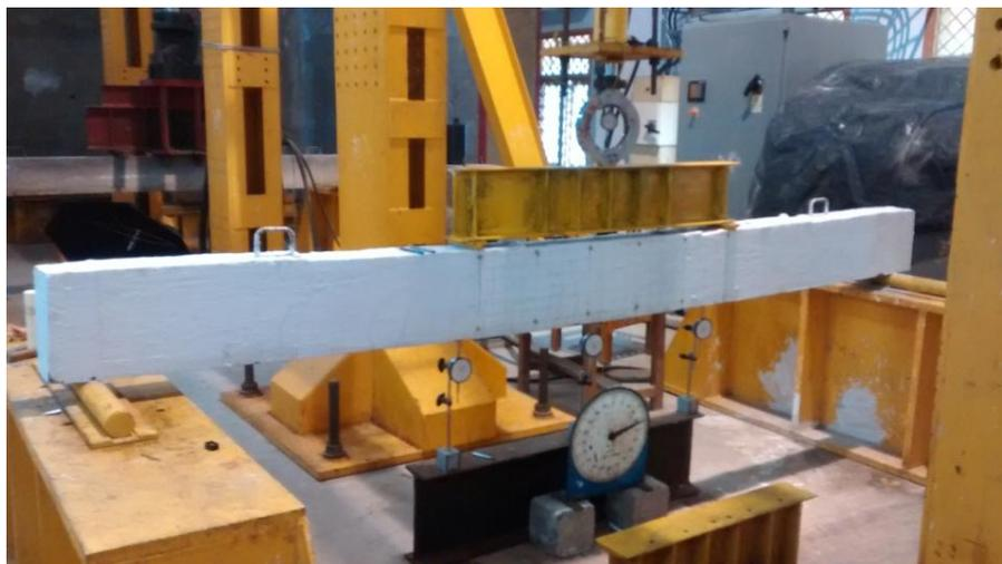
**Fig.3** Experimental Test Set-up for loading
