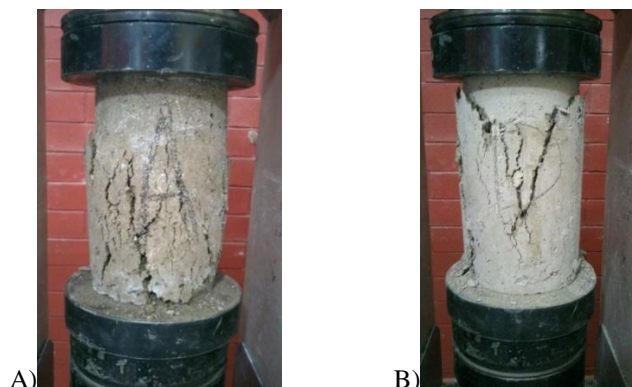
Figure 3- A) Compression of cylinder with natural latex. B) Compression of blank cylinder.
