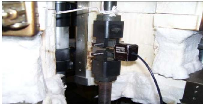
**Figure 2:** Servohydraulic Machine for CTOD Test
