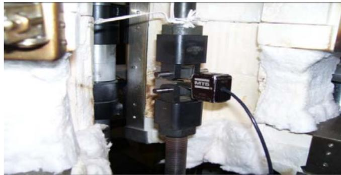
**Figure 2:** Servohydraulic Machine for CTOD Test
