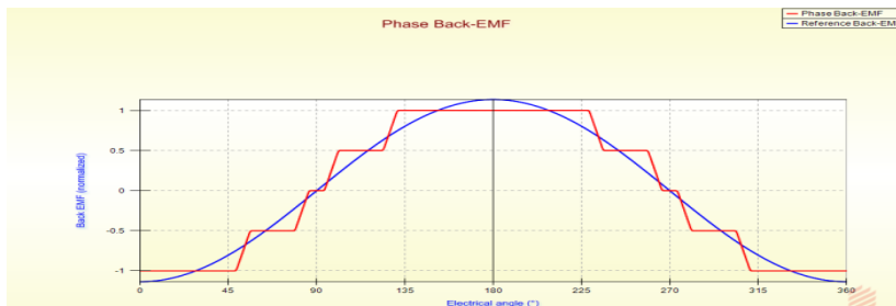
Figure 4a: phase back EMF/MMF normalized i.e. per unit value with electric pole angle of 135°
