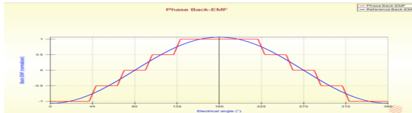
Figure 3a: phase back EMF/MMF normalized i.e. per unit value with electric pole angle of 120°
