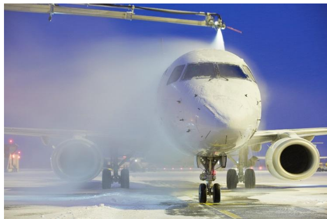
Figure 1, Ice prevention spray prior to take off.
