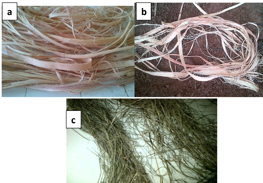
Figure 1 (a) Hand stripped fiber from the Entada mannii stalk (b) Burying of the fibers in a moist environment (c) Soil retted fibers after 20 days.
