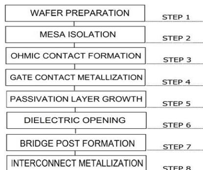
Fig. 3. Flow chart of the GaN HEMT fabrication process.
