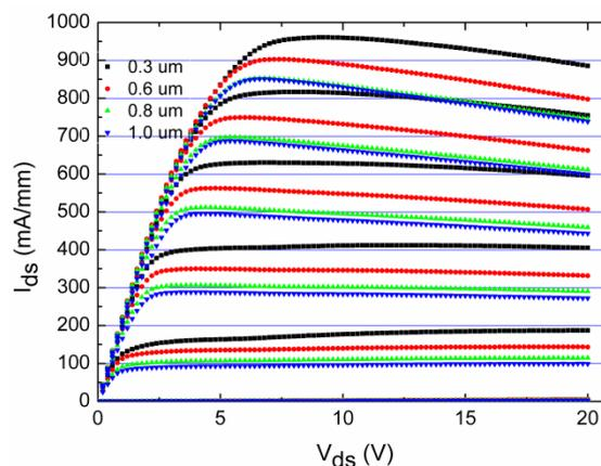
Fig. 6. Drain current-voltage ( $I_{ds}$ - $V_{ds}$ ) characteristics of a 6×125 μm AlGaIn/GaN HEMT with  $L_g = 0.3, 0.6, 0.8,$  and 1.0 μm. The gate bias was swept from +1V to -6 V in a step of -1 V.
