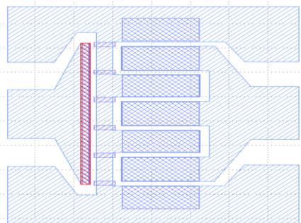
Fig. 2. Layout of an AlGaIn/GaN HEMT structure.
