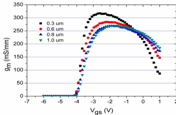
Fig. 7. Transconductance ( $g_m-V_{gs}$ ) characteristics of a  $6 \times 125 \mu\text{m}$  AlGaIn/GaN HEMT with  $L_g = 0.3, 0.6, 0.8,$  and  $1.0 \mu\text{m}$ . The gate bias was swept from  $-6$  to  $1 \text{ V}$  in a step of  $1 \text{ V}$ .
