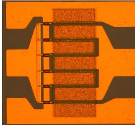
Fig. 4 Optical microscope image of fabricated 6×125μm HEMT.
