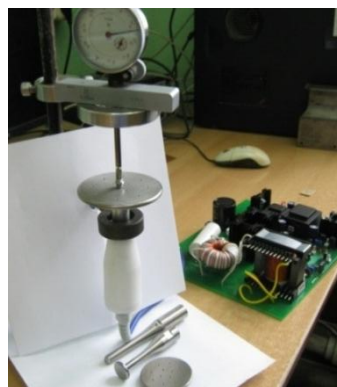
Fig. 14. Test bench for measurement of vibration amplitude of the radiating surface of the tools
