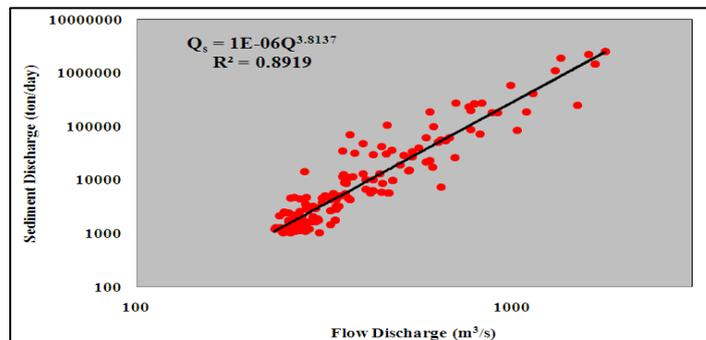
**Figure 11:** The relevance of flow discharge and sediment discharge of Karun River at upstream and Ahvaz hydrometric station
