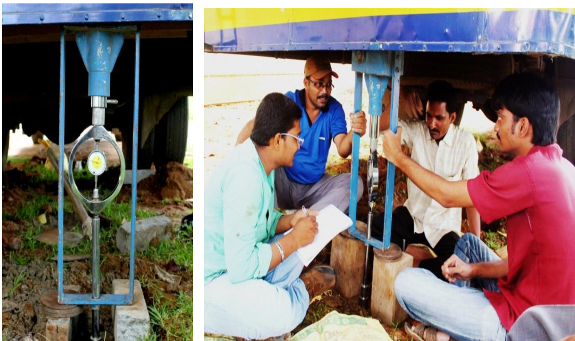
Figure III Author's performing Field CBR Test
