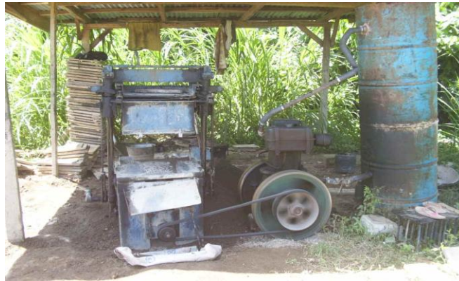
Figure 3: A diesel powered engine machine-compacted mould
