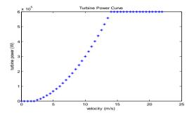
Fig.2 The output of wind turbines
