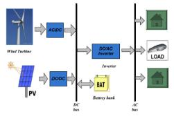
Fig. 1. Block diagram of a hybrid system.
