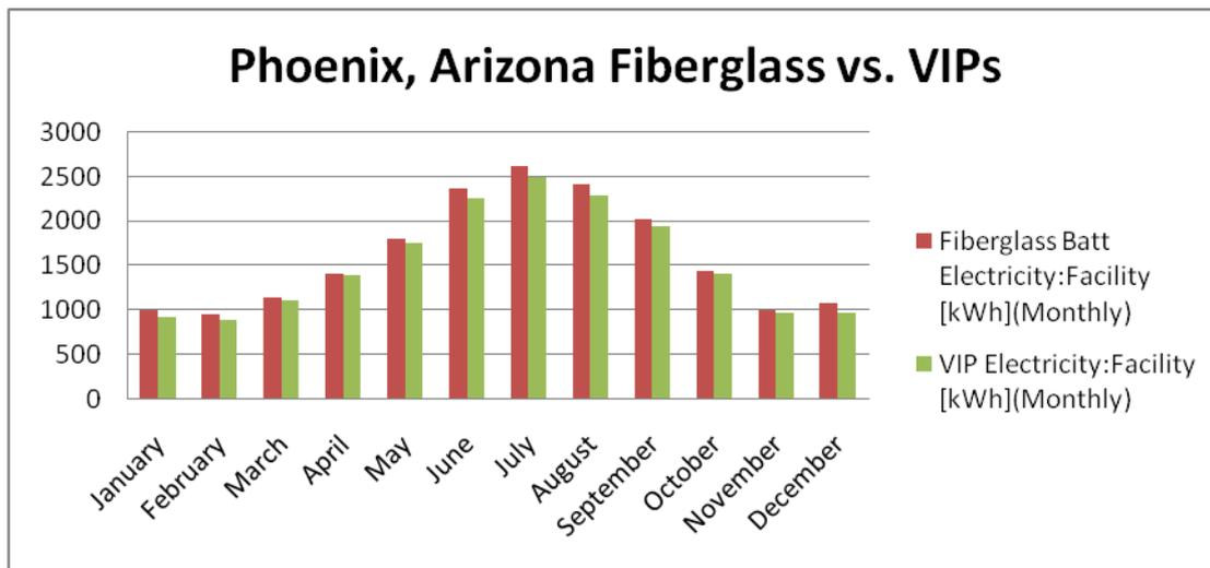
Figure 9: Results for Phoenix, Arizona, Fiberglass vs. VIPs
