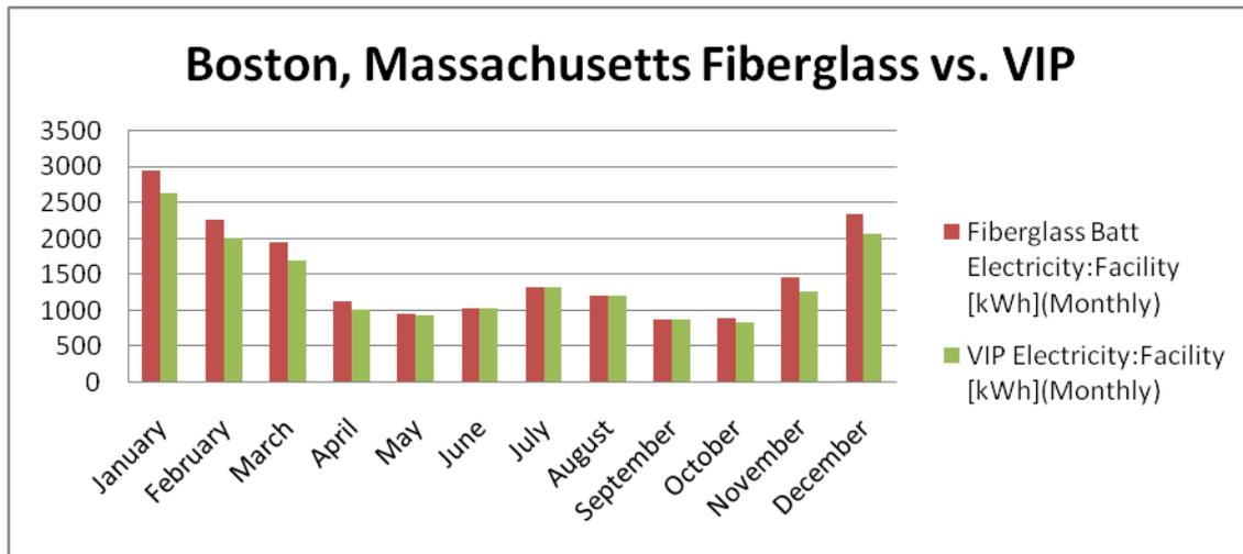
Figure 5: Results for Boston Massachusetts Fiberglass vs. VIP
