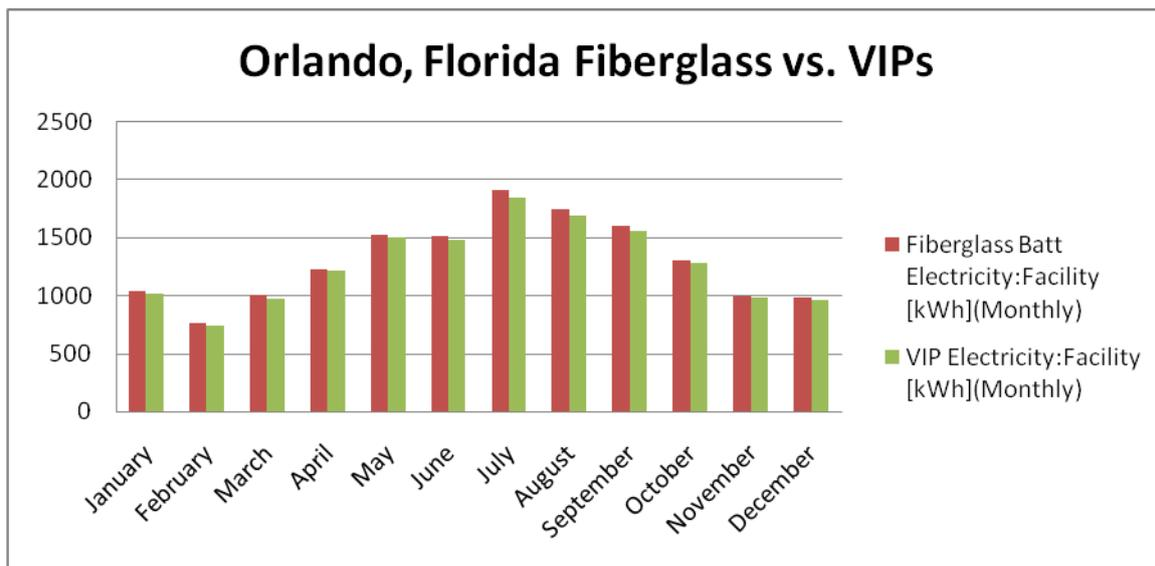
Figure 7: Results for Orlando, FL, Fiberglass vs. VIPs
