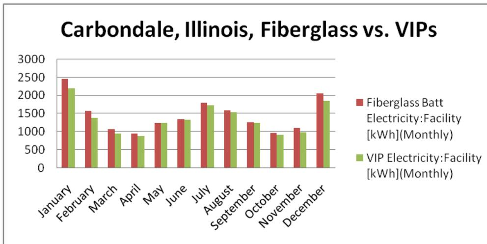
Figure 3: Results for Carbondale, Illinois, Fiberglass vs. VIPs
