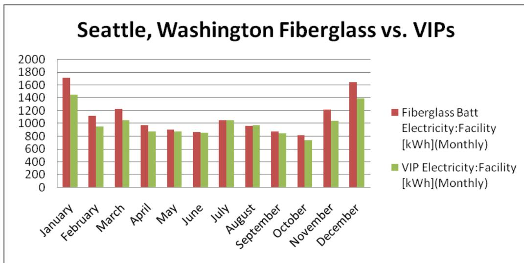
Figure 11: Results for Seattle, Washington, Fiberglass vs. VIPs
