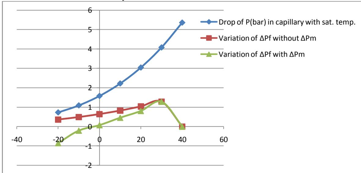
Fig-4. Actual pressure (bar) variation & elementary frictional pressure drop considering with and without momentum gain vs saturation temperature (°C) drop plots.
