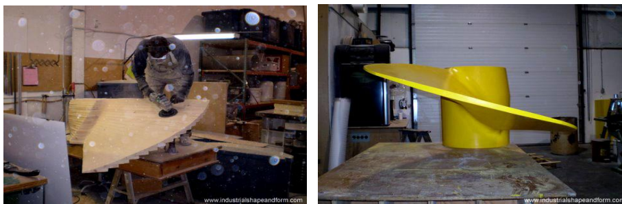
Figure 3. Shaping stack of offset wood layers and the final shape
