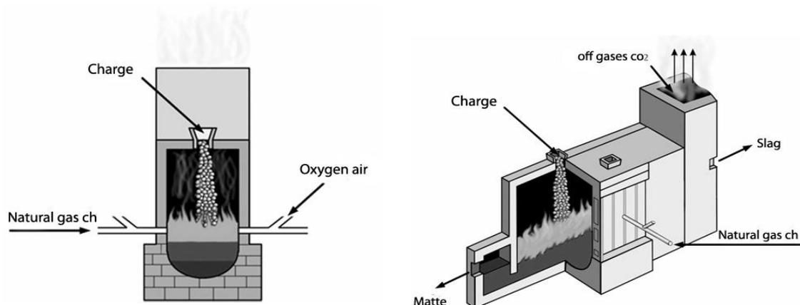
Fig. 1. Oven Vanyukov sectional
