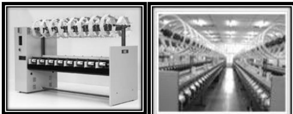
Fig. 2 spooling head of 16 spindles Fig.3 typical spooling machines
