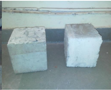
Figure 2 Cement concrete cubes in wet and dry state
