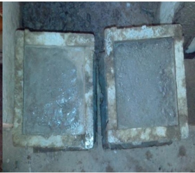
Figure 2 Cement concrete cubes in wet and dry state
