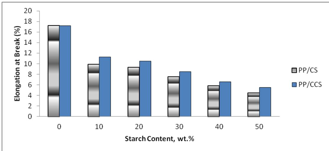
Fig. 6: Elongation at Break of PP/CS Blends
