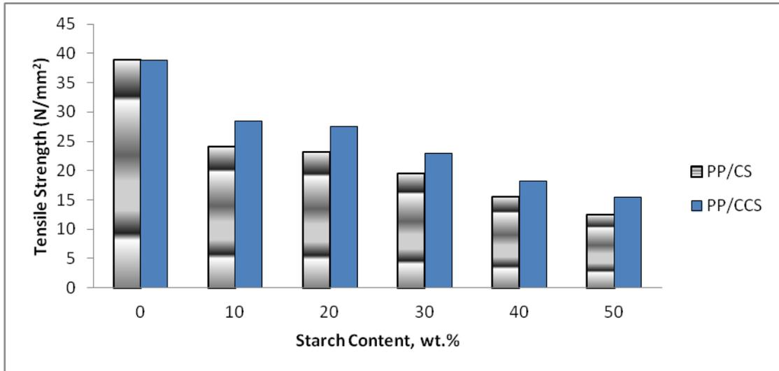
Fig. 5: Tensile Strength of PP/CS Blends
