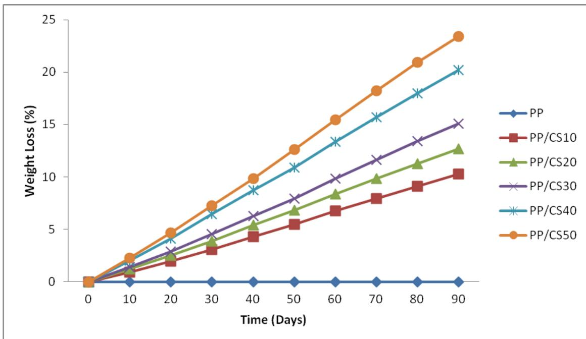
Fig. 3: Weight Loss for PP/CS Blends
