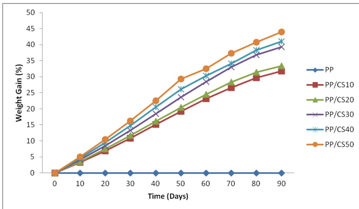
Fig. 1: Water absorption for PP/CS Blends
