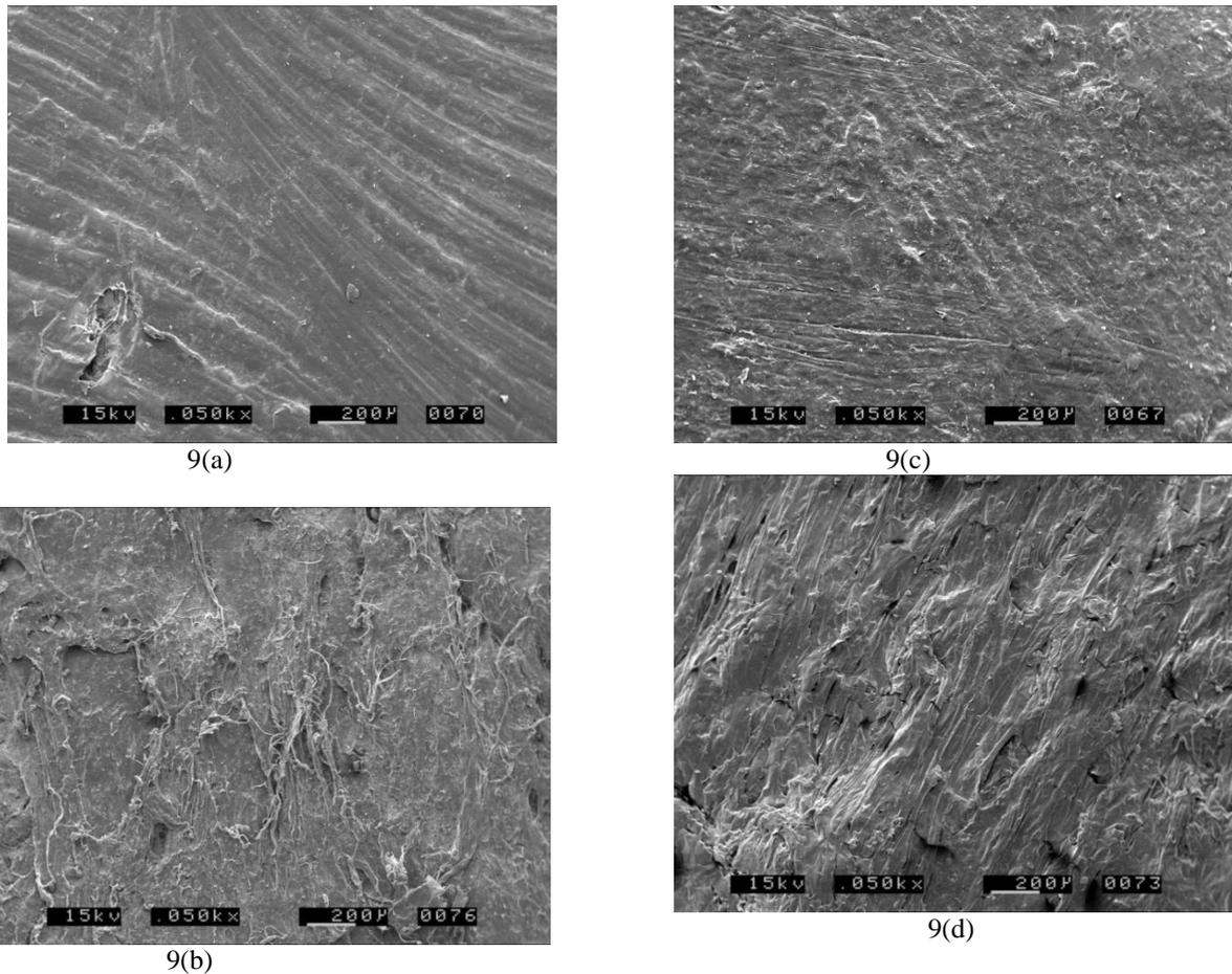
Fig. 9: SEM images of PP/CCS blends, (a) 10 % CCS and (b) 50 % CCS before soil burial; (c) 10 % CCS and (d) 50 % CCS after soil burial.
