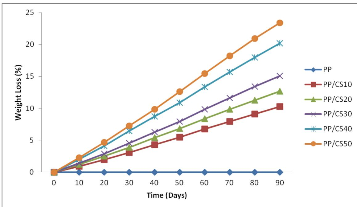
Fig. 3: Weight Loss for PP/CS Blends
