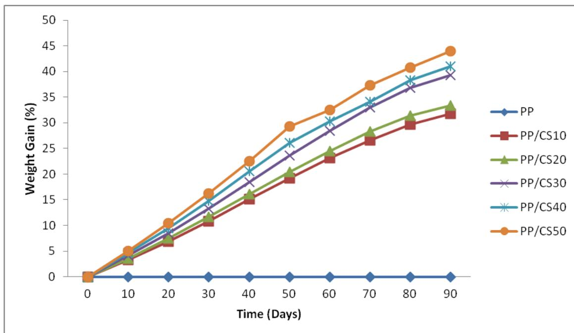
Fig. 1: Water absorption for PP/CS Blends
