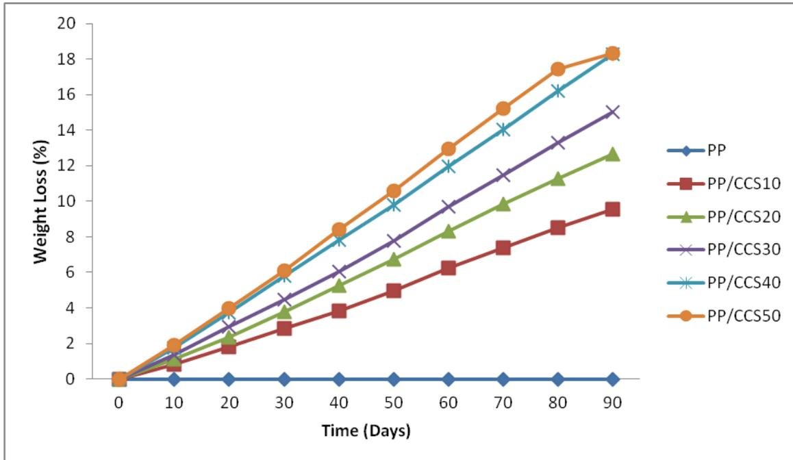
Fig. 4: Weight Loss for PP/CCS Blends
