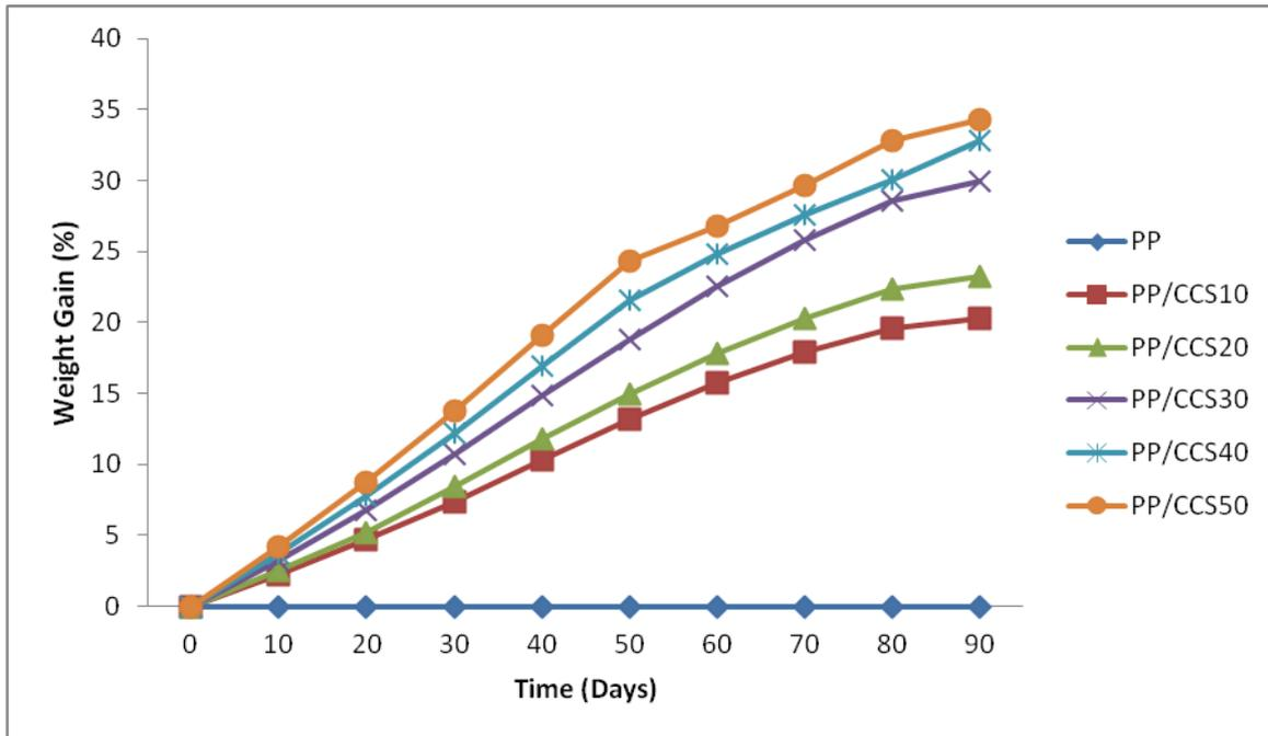
Fig. 2: Water absorption for PP/CCS Blends
