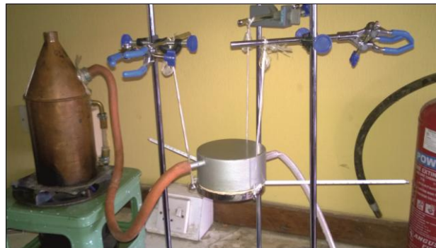
A3: Experimental Set-up of Lee-Charnton's Method in Determination of Thermal Conductivity
