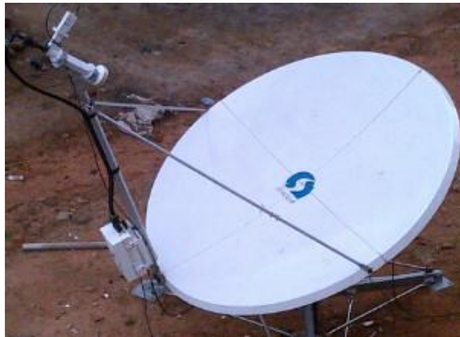
Figure 4.1: 1.2M C-Band Satellite Antenna for Outdoor STV Broadcast [22]
