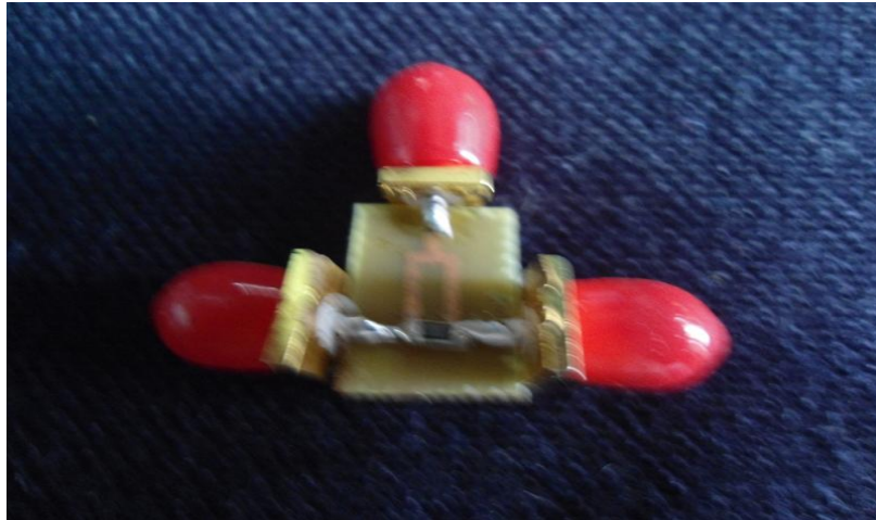
Fig.3 fabricated Structure of Proposed WB Power Divider (Dimension is 15 mm×10.3 mm)
