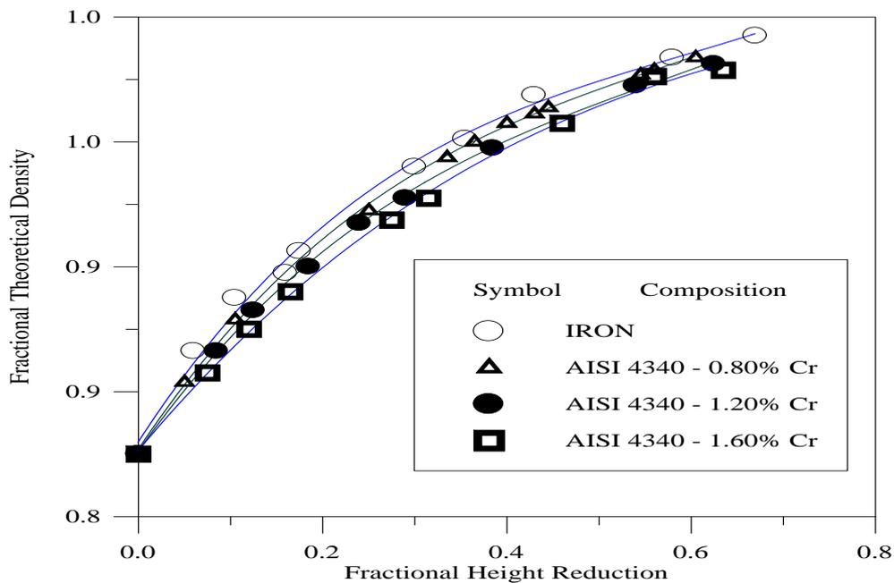
**Figure 2 Relationship Between Fractional Density and the Fractional Height Reduction During Hot Forging of Sintered P/M Steel Ring Preforms of Initial Preform Geometry.**
