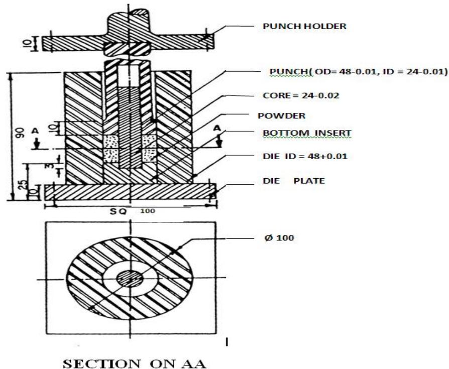
Figure 1 Die Assembly for Compaction of Powder Preforms
