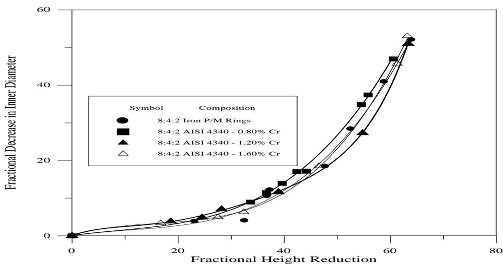
**Figure 3 Relationship between Fractional Inner Diameter Decrease and Fractional Height Reduction of 8:4:2 Ring geometry Preforms of Sintered P/M Steels during Hot Upset Forging**
