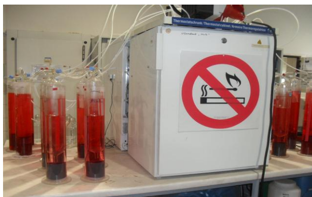
Plate 1: Experimental set up for batch digestion
