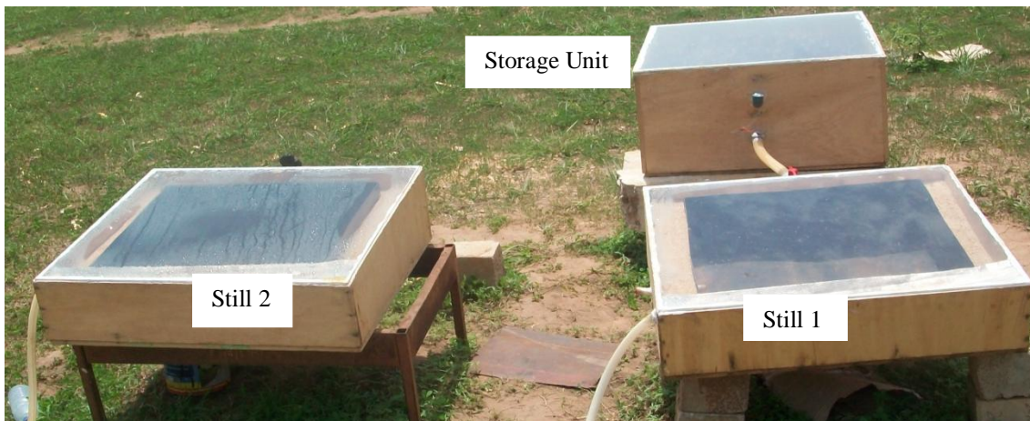
Plate 1: picture of the components of the set up for the study
