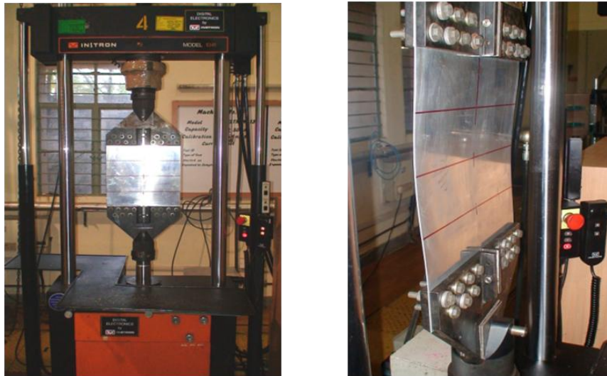
Figure 2: Buckling test setup and onset of buckling in square aluminum plate
