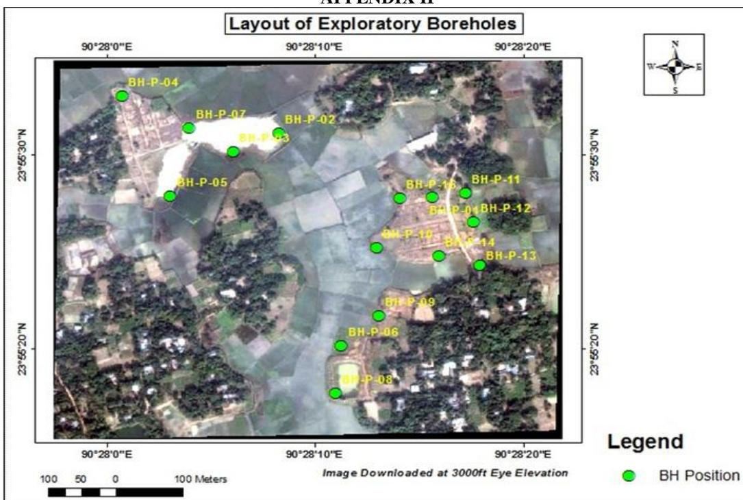
Figure 9. Exploratory boreholes layout map.
