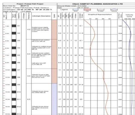
Figure 10. Log sheets of the 15 SPT boreholes completed at Prabasi Palli
