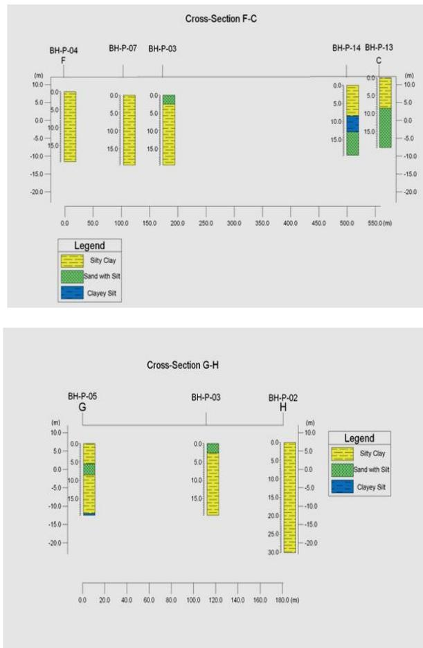
Figure 5. Presents litho logs and geological and cross-sections obtained from the boreholes.
