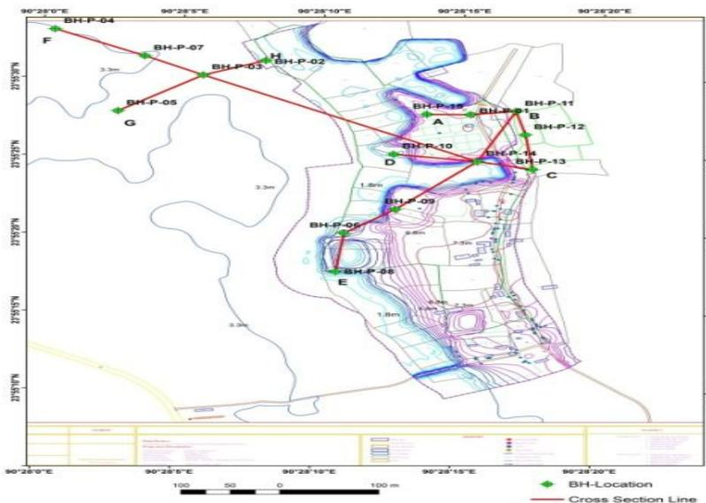
Figure 11. Map showing lines A-B, B-C, C-D, D-E, E-F and F-G taken for geological Cross-sections as in figure 5.
