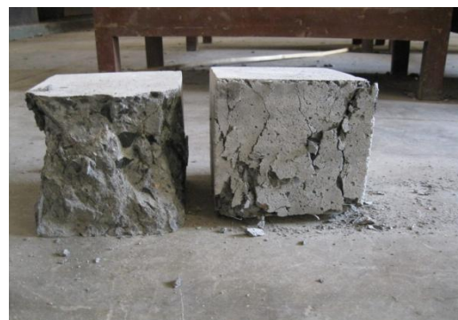
Photograph 2 Tested specimens of normal and PFRC
