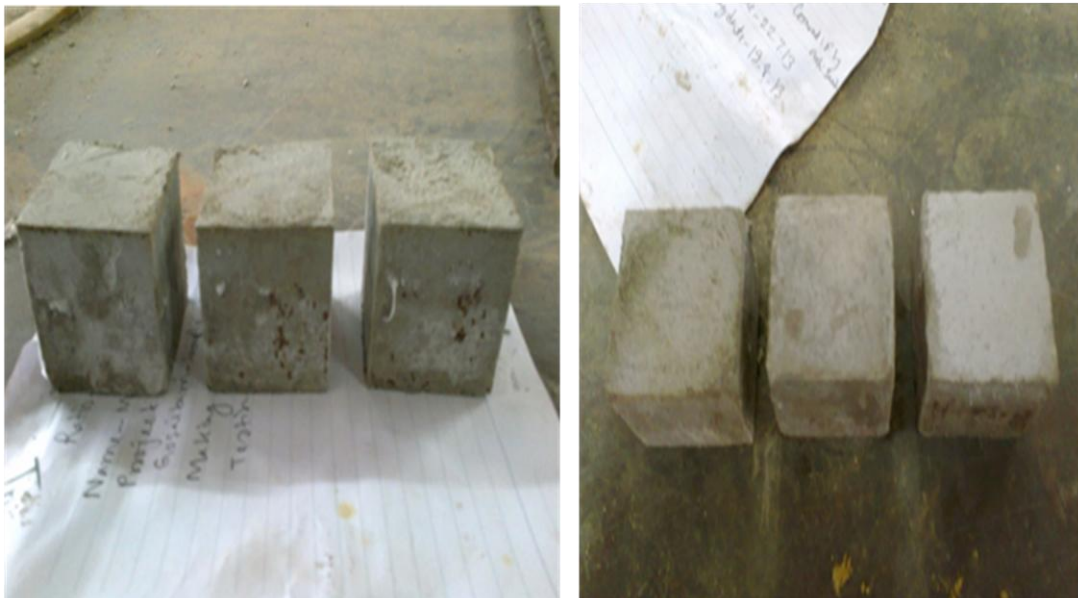
Figure 6. Some samples of backfill material with different ratio of cement: fly ash: sand
