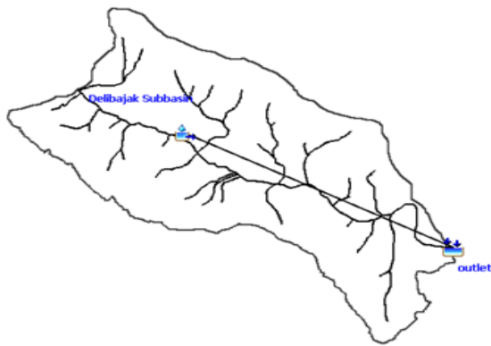
Fig 2. Processed results for Lumped Delibajak basin imported to HEC- HMS for simulation
