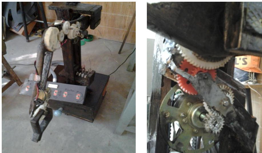
Fig. 9 increasing torque by adding external gear
