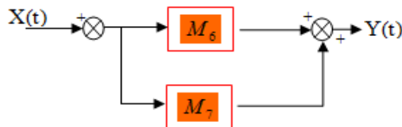
Figure (5). The transformation of the structure of the block diagram of transfer to sub-models for winding coils with the finished yarn
