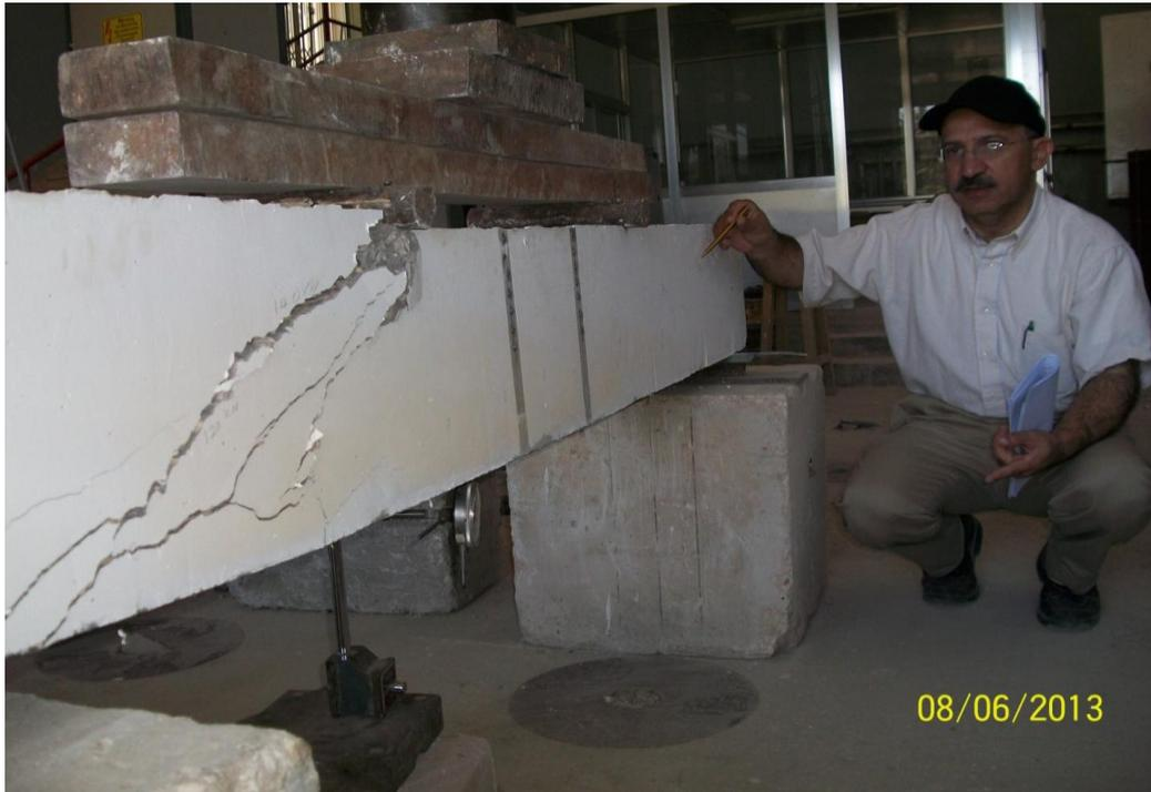
Figure 6: Beam BU at failure stage
