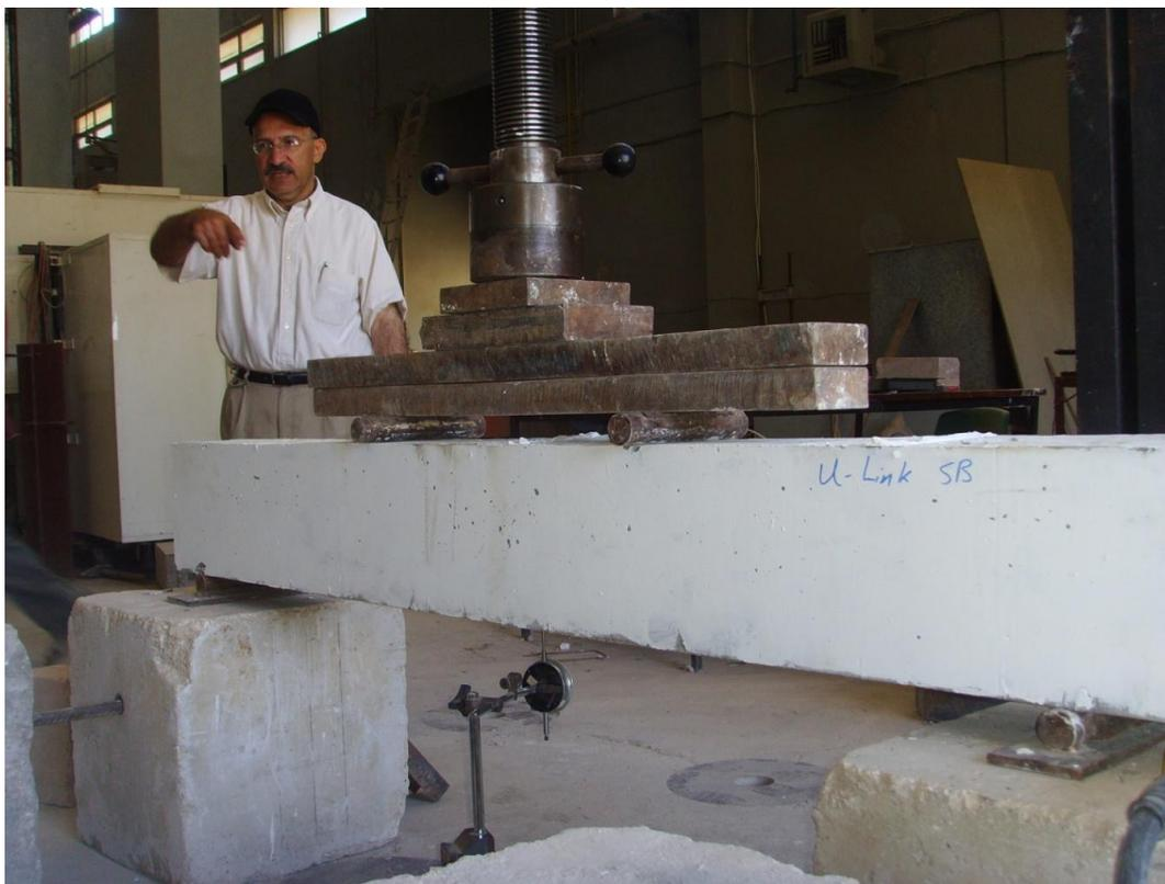
Figure 5: Experimental set up and crack monitoring
