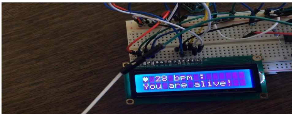
Figure 5.1. Displaying ECG signals on the LCD screen
