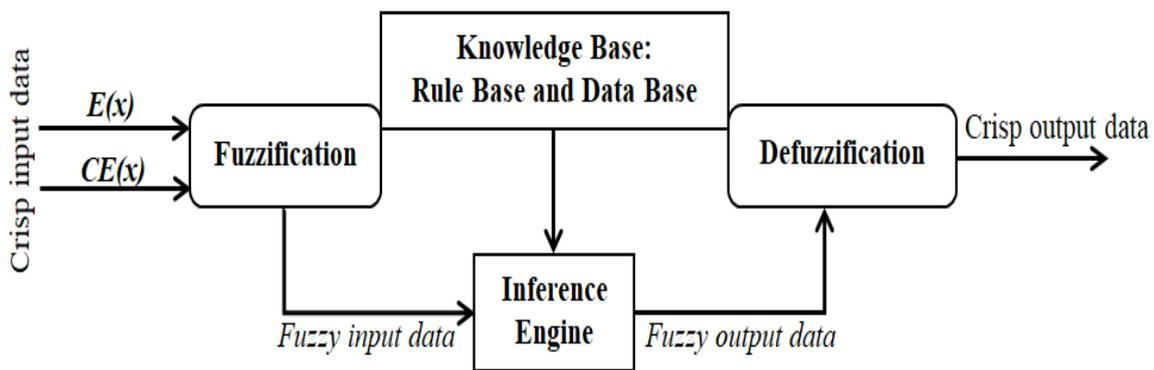
Figure 4: The Structure of a fuzzy logic control system
