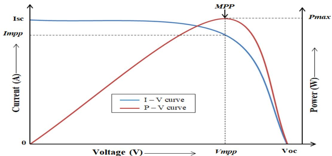
Figure 1: Solar cell I – V and P – V characteristics
