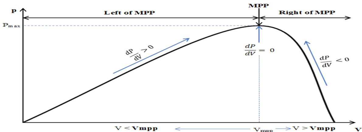
Figure 2: Operating Principle of perturbation and observation in P-V curve
