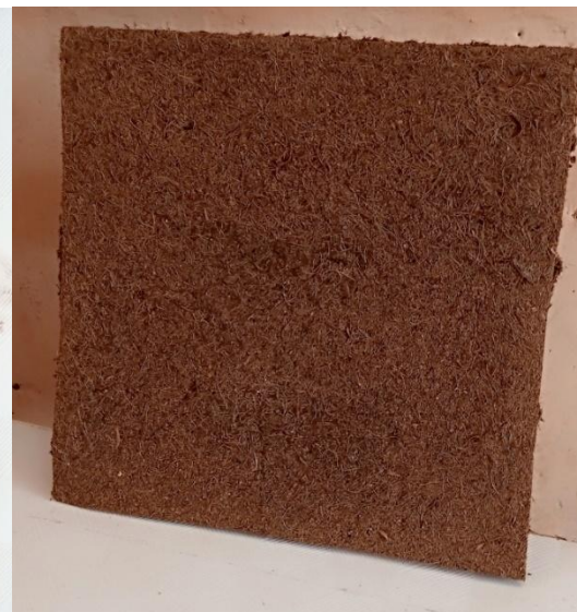
Fig 6. Bio- composite of Ground nut shell and Palm kernel Ceiling Board
