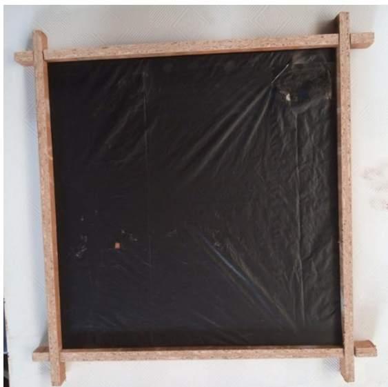
Fig. 5. 400x400x12mm wooden mould
