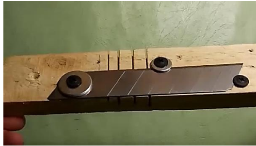
Fig.2. Instrument for manufacturing PET threads of different widths.
