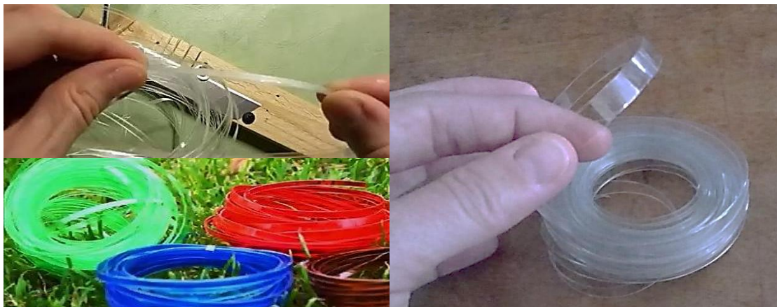
Fig.3. PET thread that is obtained after the spinning process.
