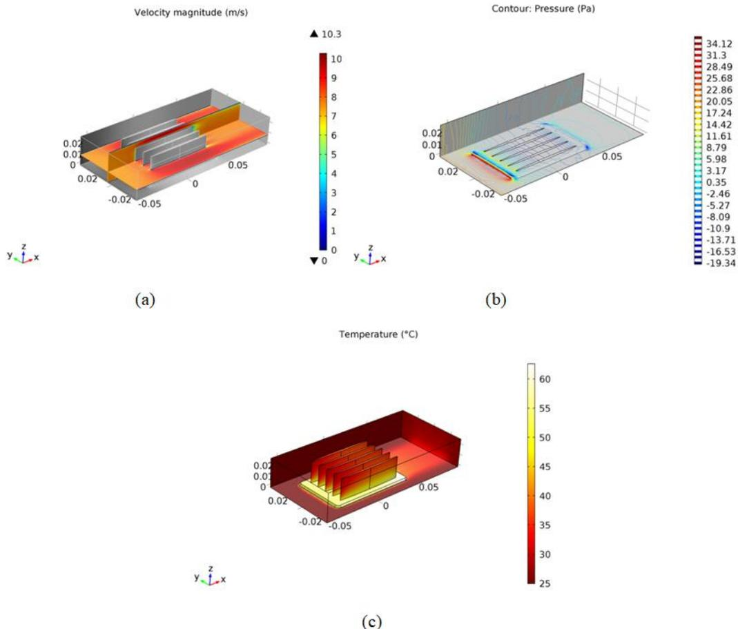
**Fig 5.** Results from the airfoil-shaped titanium heat sink a) Velocity b) Pressure c) Temperature
