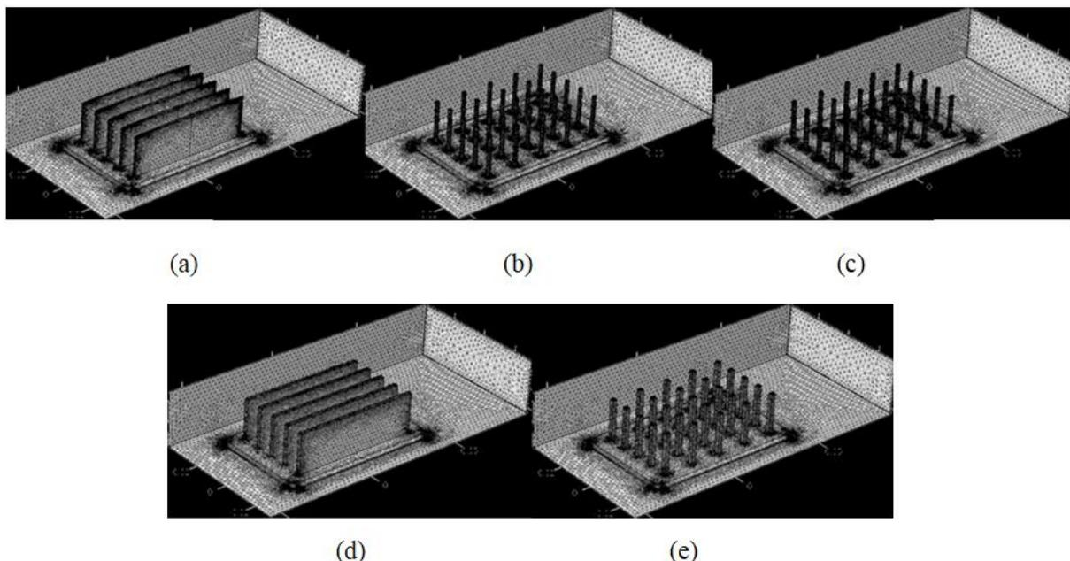
**Fig 2.** Heat sink configurations used in COMSOL software a) Airfoil b) Pin Hexagonal c) Pin Squared) Rectangular e) Pin Circular
