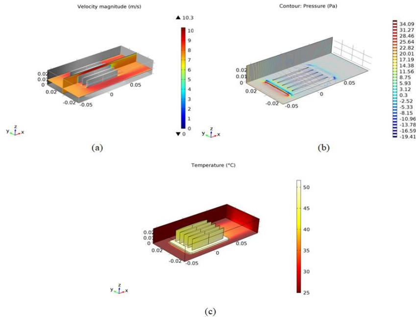
**Fig 3.** Results from the airfoil-shaped aluminum heat sink a) Velocity b) Pressure c) Temperature
