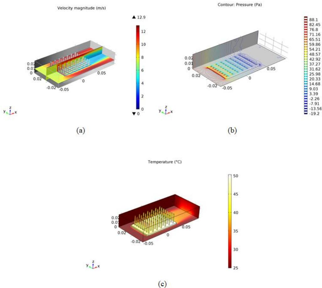
**Fig 4.** Results from the pin circular-shaped aluminum heat sink a) Velocity b) Pressure c) Temperature
