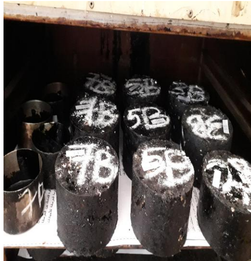
Fig. 4: The specimens at oven for five days at 85°C
