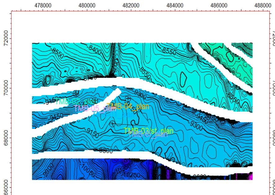
Figure 7: Sand F-Subsurface Map (Depth)
